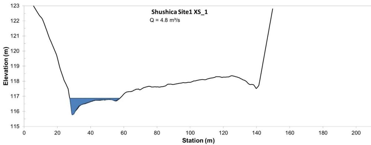
Figure 5. Cross-section XS\_1 including measured water level at a discharge of  $4.8 \text{ m}^3/\text{s}$
