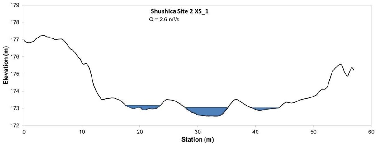
Figure 11. Cross-section XS\_1 including measured water level at a discharge of  $2.6 \text{ m}^3/\text{s}$
