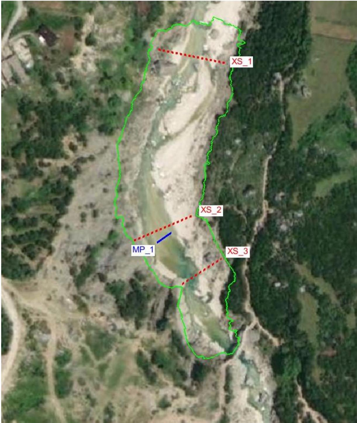
Figure 8. Aerial view of Shushica site 2; MP = measurement Profile (blue line); XS=cross-section (dashed red line); green polygon = DTM boundary
