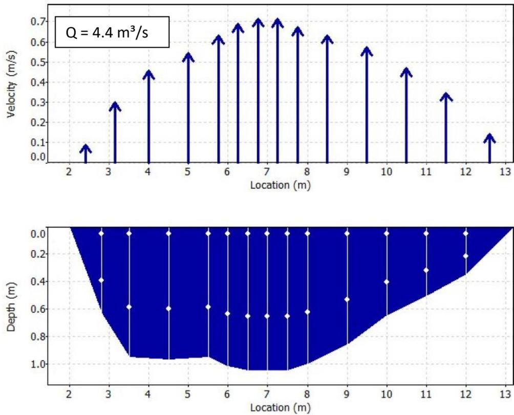
Figure 4. Measured mean flow velocity (top) and measurement profile MP\_3 (bottom) at Shushica 1.
