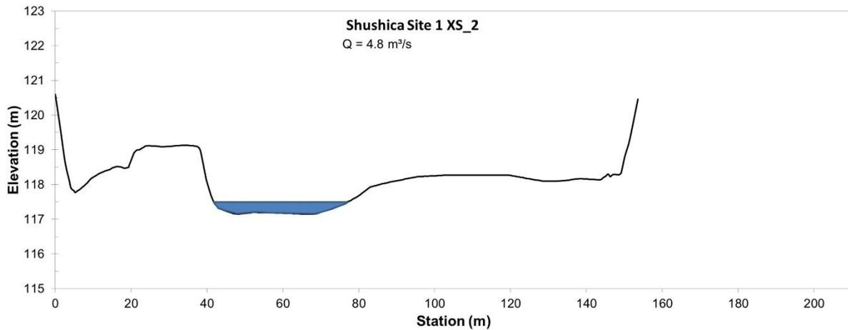
Figure 6. Cross-section XS\_2 including measured water level at a discharge of  $4.8 \text{ m}^3/\text{s}$
