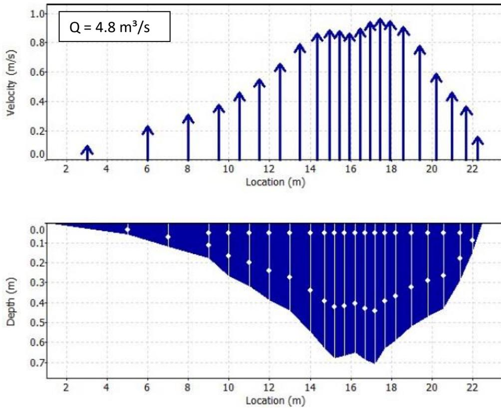
Figure 2. Measured mean flow velocity (top) and measurement profile MP\_1 (bottom) at Shushica 1.
