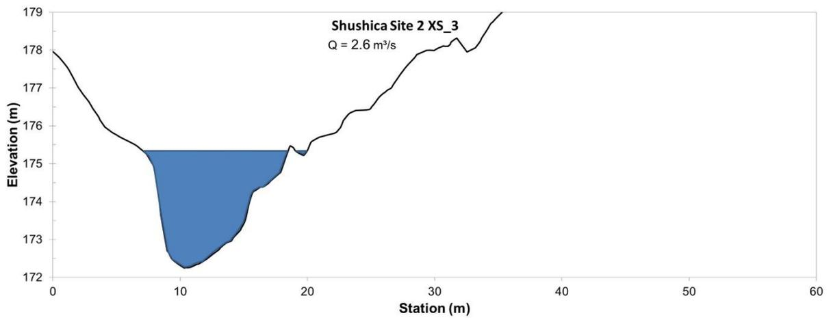
Figure 13. Cross-section XS\_3 including measured water level at a discharge of 2.6 m<sup>3</sup>/s
